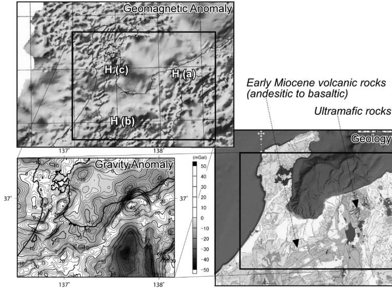
**Figure 1.4** Geomagnetic anomaly trend around the Hokuriku Province (Nakatsuka and Okuma, 2005) together with Bouguer gravity anomaly (Komazawa, 2004) and geologic (Geological Survey of Japan, 2012) maps. Annotation 'H' in geomagnetic anomaly map corresponds to area accompanied by remarkable high (positive) anomaly.
